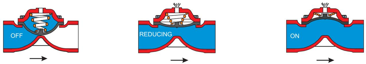
Hydraulic control valves are direct - sealing diaphragm valves activated by pipeline pressure. When in the control chamber pressure is equal to the pipeline pressure the rubber diaphragm closes the valve. The spring in the upper side of diaphragm helps valve to close regardless of pressure and flow conditions. Expanding the pressure from control chamber ,valve opens. The valve's only moving part is its diaphragm.
