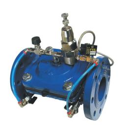
PRE - V valve reduces the upstream pressure in a defined downstream pressure, regardless of pressure and flow-rate fluctuations, opens and closes with a solenoid valve.
